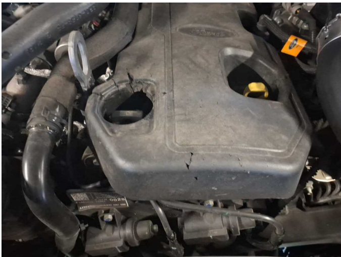
Damage 10: Engine: Engine cover - Damage caused by martensite / rodent - Replace
