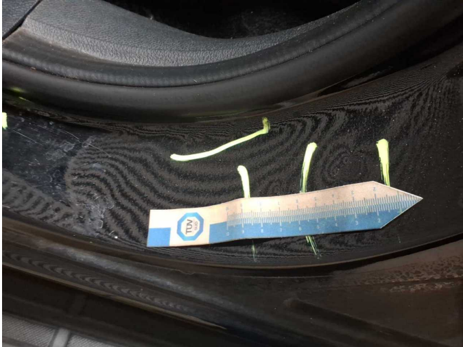
Damage 9: Sill - left side: Sill - dent(s) - Smooth repair work
