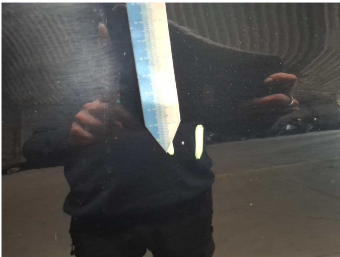
Damage 8: Side panel - rear right side: Side panel - Stone chips - Smart repair
