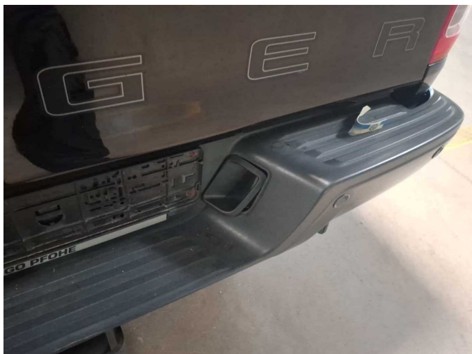
Damage 3: Tail light: License plate lamp - right side (Halter) - Loose - Replace
