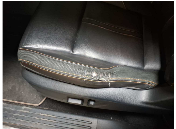
Damage 11: Seat - front: Seat cover - left side - Broken / torn - Replace
