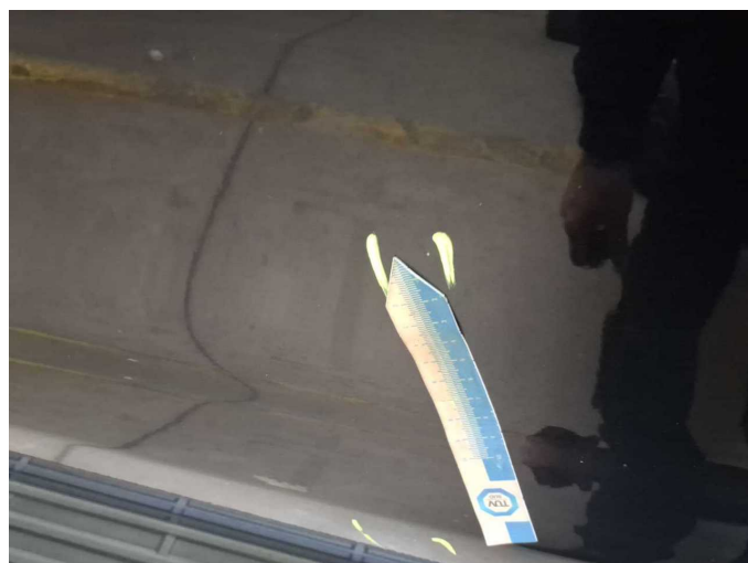
Damage 12: Door - rear left side: Door - Scratched - Paint
