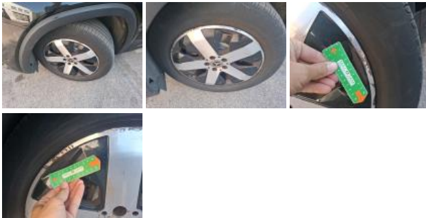
Tyre RL, Out of tolerance, Replace
