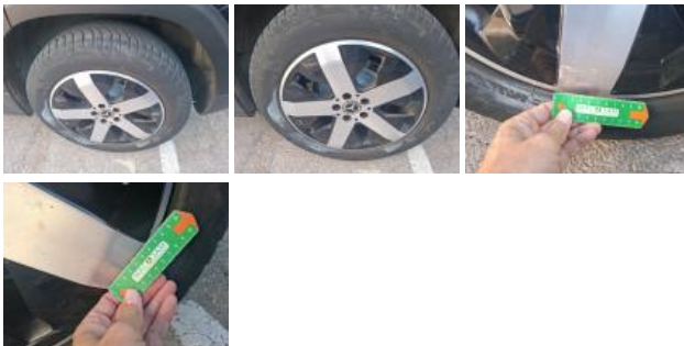
Tyre RR, Out of tolerance, Replace
