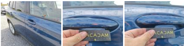
Bodywork, Paint measurement, Acceptable
