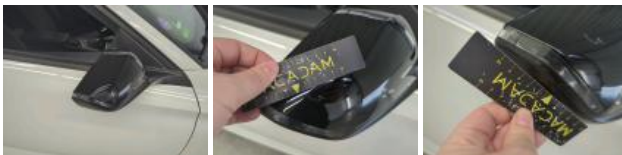
Mirror side repeater R, Scratch(es), Replace
