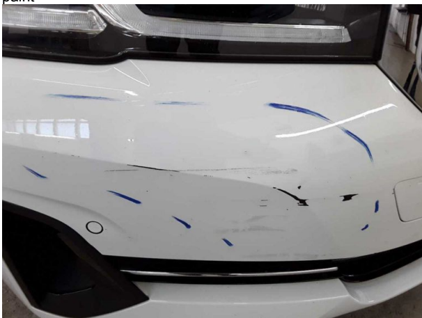
Damage #9: Front bumper: Bumper with Parktronic - Scratched - Repair and paint
