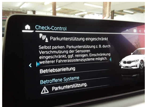
Damage #5: Electronic systems: Parking assistance (Fehlermeldung) - Specify findings - Perform diagnosis
