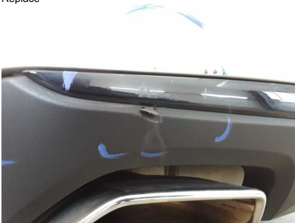
Damage #7: Rear bumper: Spoiler - Deformed - Replace
