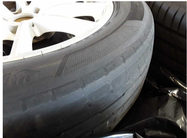
Damage #3: Measurement: Undercarriage - Malposition - Set / adjust
