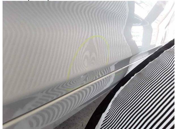
Damage #11: Door - front left side: Door - dent(s) - Repair and paint
