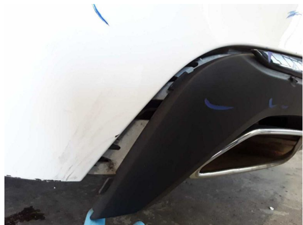
Damage #7: Rear bumper: Spoiler - Deformed - Replace
