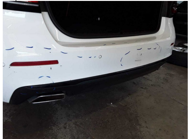
Damage #7: Rear bumper: Spoiler - Deformed - Replace
