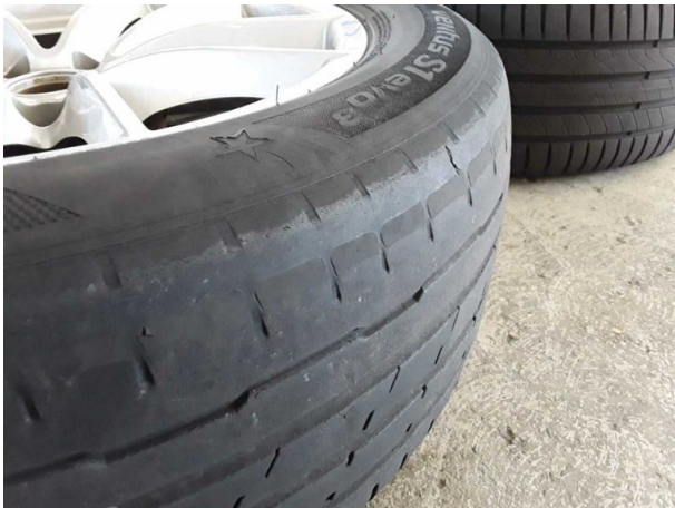
Damage #3: Measurement: Undercarriage - Malposition - Set / adjust
