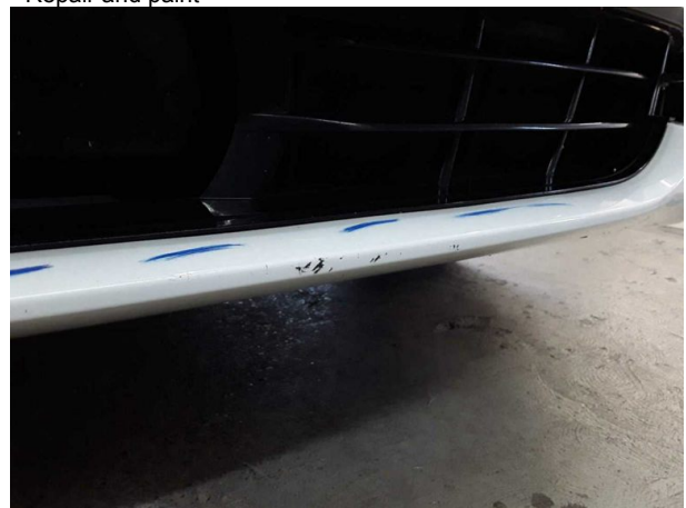
Damage #9: Front bumper: Bumper with Parktronic - Scratch... - Repair and paint
