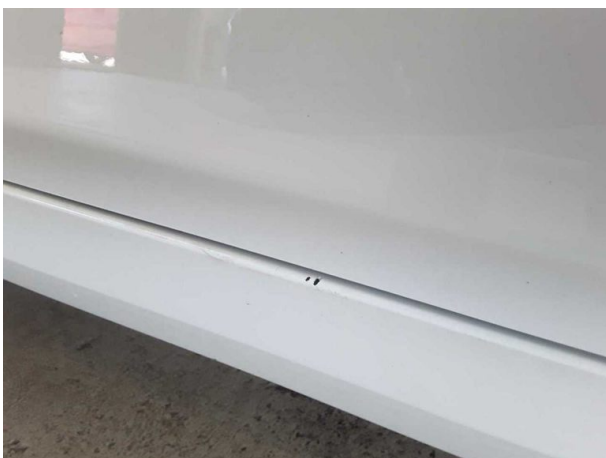
Damage #4: Sill - left side: Trim - Scratched - Smart repair
