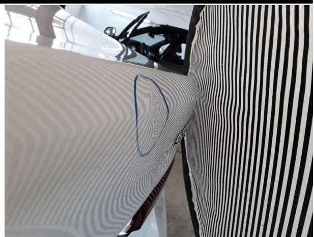
Damage #8: Boot lid / rear door: Boot lid - dent(s) - Repair and paint
