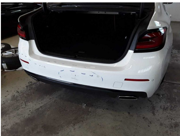
Damage #12: Rear bumper: Bumper with Parktronic - Deformed - Replace
