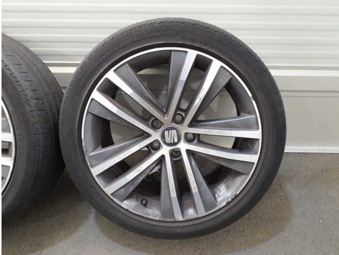
Damage 2: 2nd wheel set: 1 tyre - Porous / cracked - Replace
