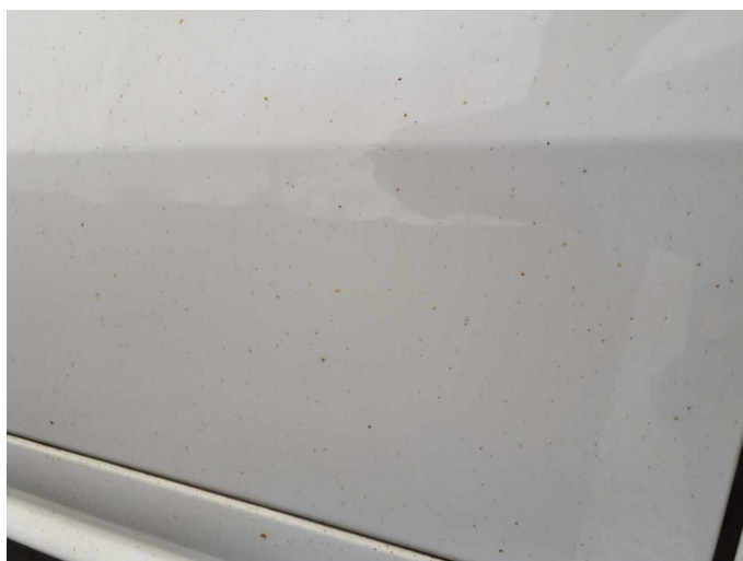
Damage 4: Body: Body (Flugrost) - Soiled - Clean
