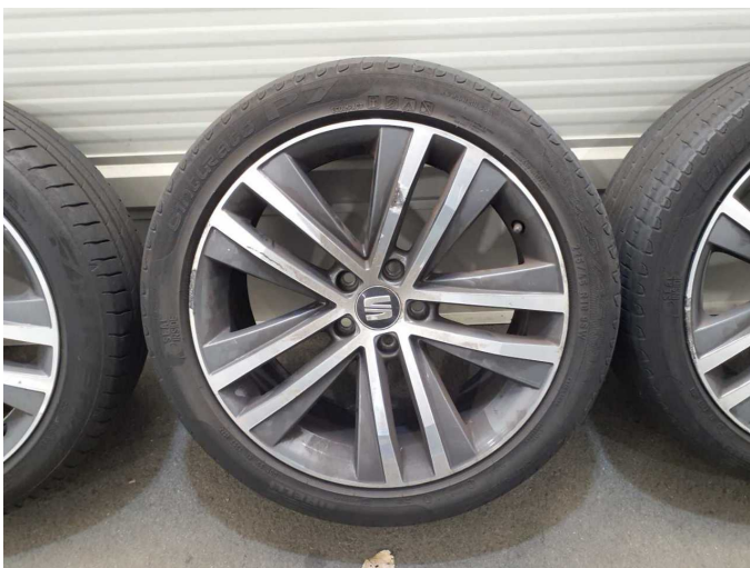
Damage 3: 2nd wheel set: 1 tyre - Porous / cracked - Replace
