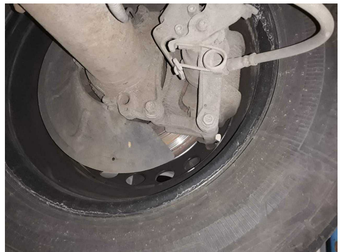
Damage 7: Braking system: Brake discs and pads - rear - Corrosion - Replace
