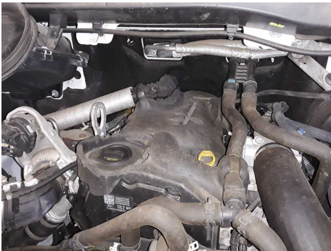
Damage 6: Engine: Engine cover - Broken / torn - Replace
