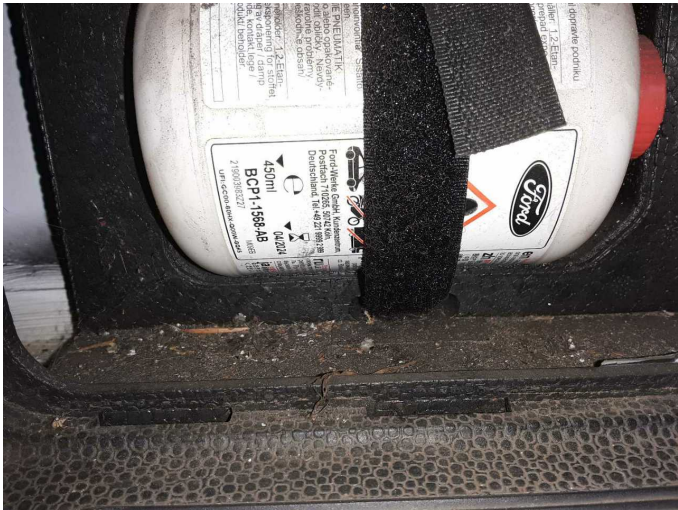
Damage 1: Equipment: Tirefit filler - Due - Replace
