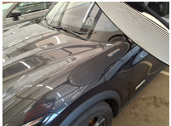
Damage 2: Mudguard - left side: Mudguard - left side - dent(s) - Smooth repair work
