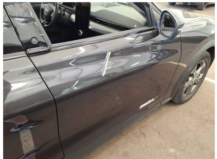
Damage 3: Door - front right side: Door - Dent / paintcoat damage - Repair and paint
