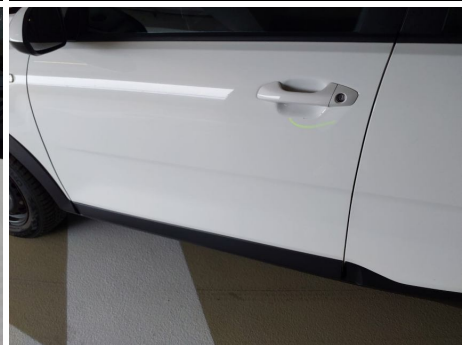
Tür / Vorne Links / Kratzer
