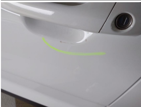
Tür / Vorne Links / Kratzer
