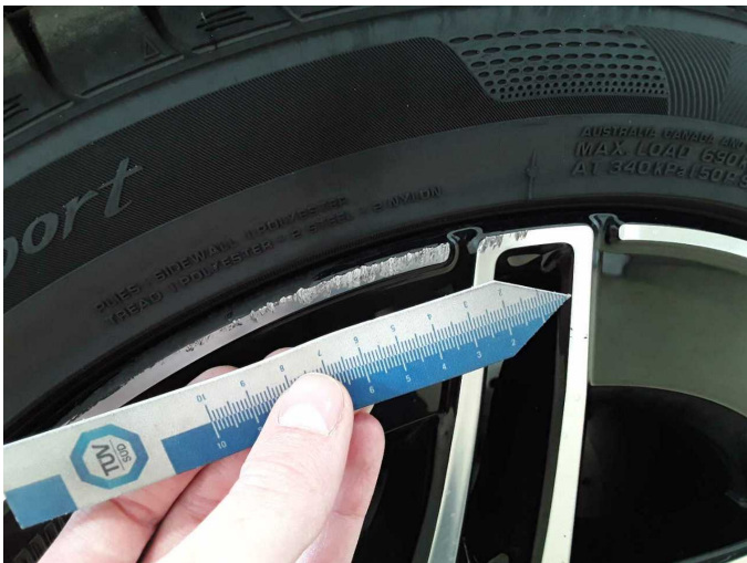
Damage 5: Wheel / tyres: Alloy rim - front right side - Scratch(es) - Replace
