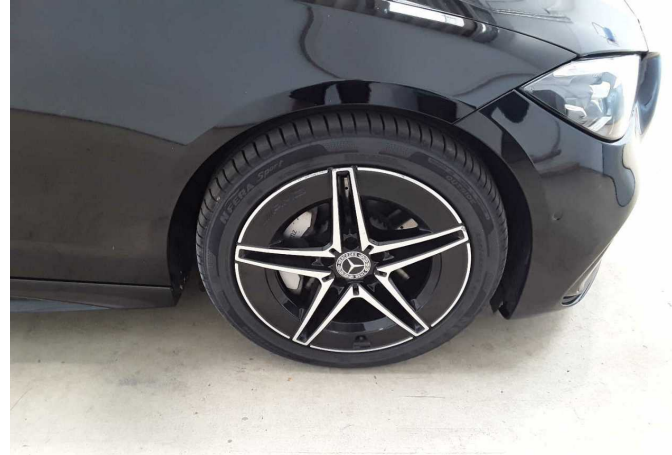
Damage 5: Wheel / tyres: Alloy rim - front right side - Scratch(es) - Replace
