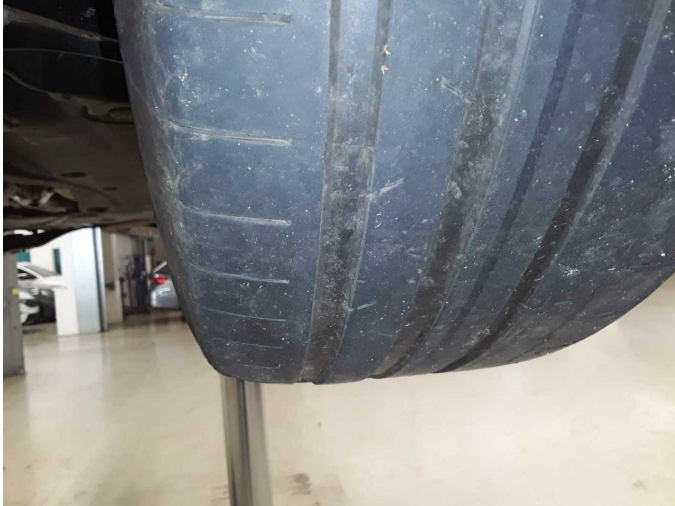
Damage 8: Wheel / tyres: Tyre - front - does not meet manufacturer specifications - Replace
