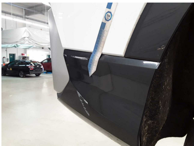
Damage 12: Rear bumper: Rear bumper (Incl. Anbauteile erneuern) - Scratched - Repair and paint
