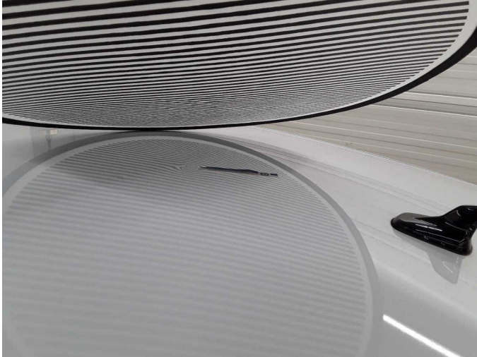
Damage 5: Roof: Roof - dent(s) - Smart repair
