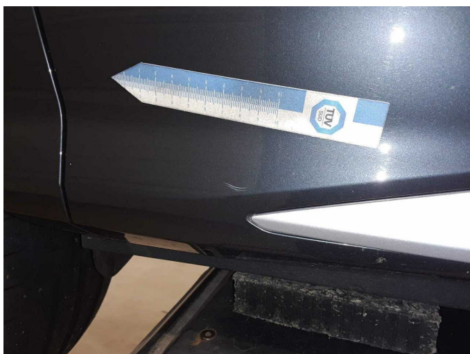
Damage 3: Door - rear right side: Brightware - lower - Scratch(es) - Smart repair
