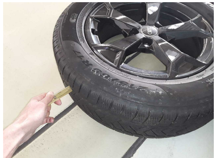
Damage 7: 2nd wheel set: 2 tyres - does not meet manufacturer specifications - Replace
