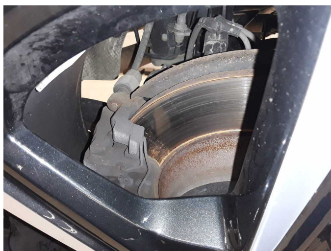
Damage 10: Braking system: Brake discs and pads - rear - Worn - Replace
