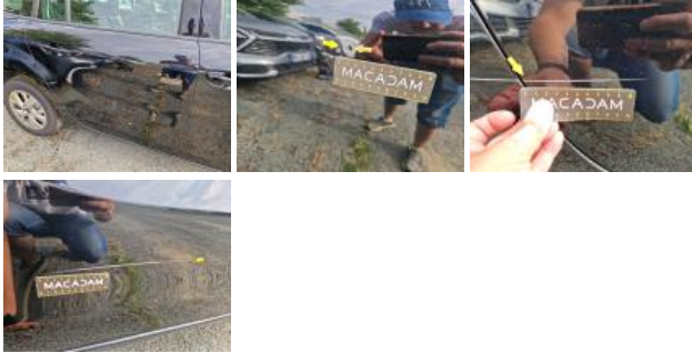
Outer sill R, Dent(s) and scratch(es), Repair and paint (complete)
