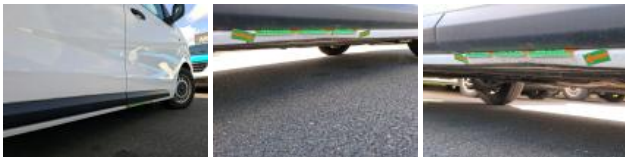
Outer sill R, Dent(s) and scratch(es), Repair and paint (complete)
