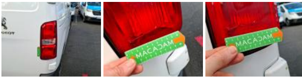
Boot door panel RR, Dent(s), Repair and paint (complete)
