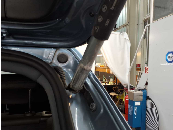
Damage 5: Boot lid / rear door: Gas pressure damper - Broken / torn - Replace
