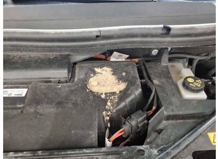
Damage 1: Air-conditioning system: Air-conditioning system (Isolierung Klimagehäuse) - Damage caused by marten / rodent - Replace
