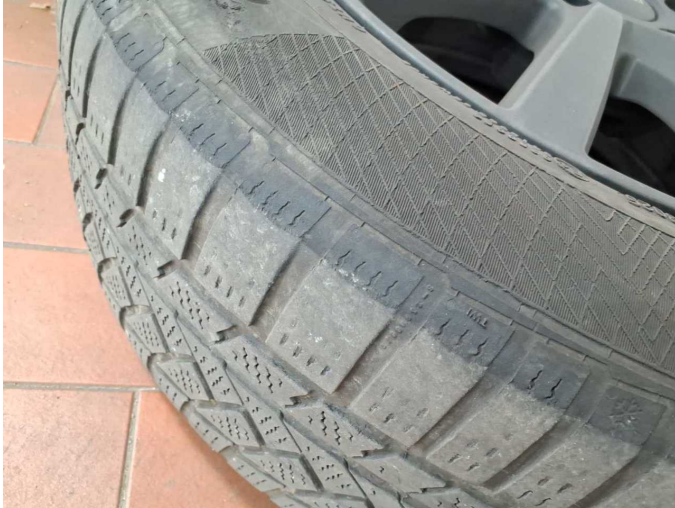
Damage 6: Wheel / tyres: Tyre - front - Abrasion - Replace
