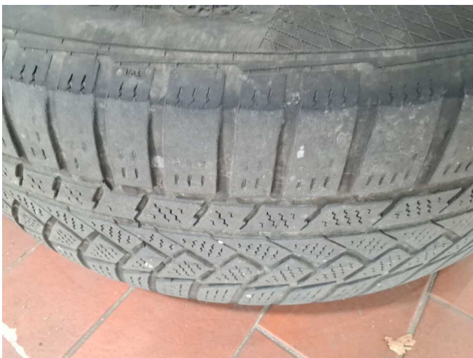
Damage 6: Wheel / tyres: Tyre - front - Abrasion - Replace
