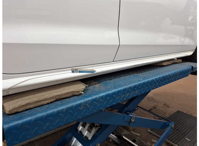
Damage 4: Sill - right side: Trim - Scratched - Paint
