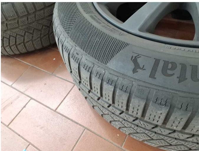
Damage 6: Wheel / tyres: Tyre - front - Abrasion - Replace
