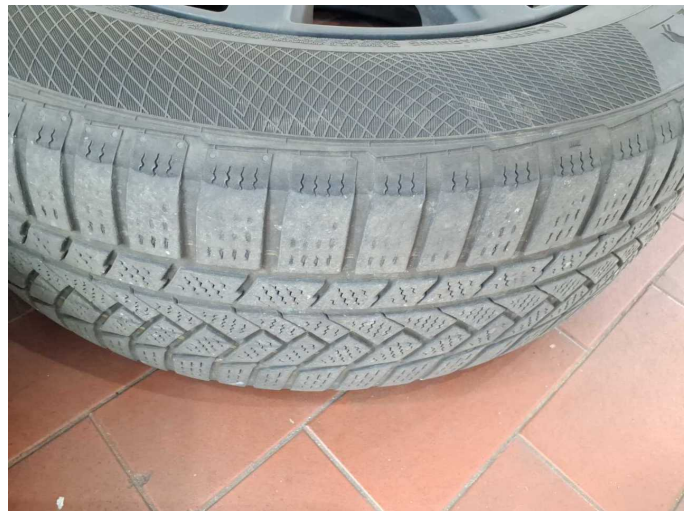
Damage 6: Wheel / tyres: Tyre - front - Abrasion - Replace
