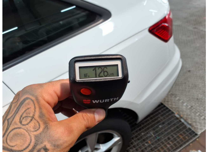
Previous damage 1: Rear, Side - left
