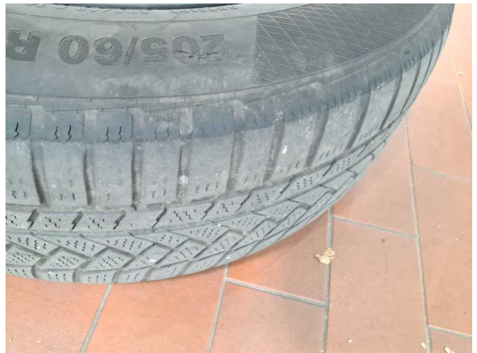
Damage 6: Wheel / tyres: Tyre - front - Abrasion - Replace
