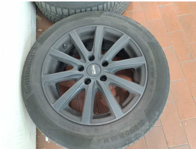
Damage 6: Wheel / tyres: Tyre - front - Abrasion - Replace
