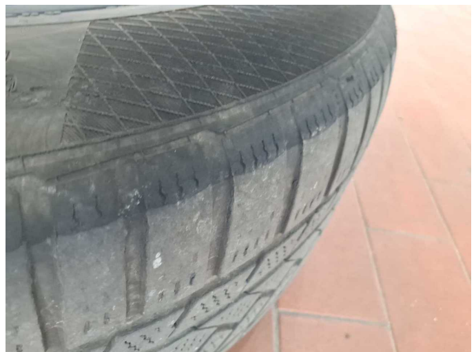
Damage 6: Wheel / tyres: Tyre - front - Abrasion - Replace
