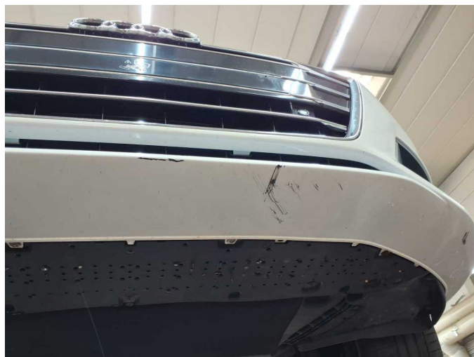
Damage 8: Front bumper: Front bumper - Scratched - Paint
