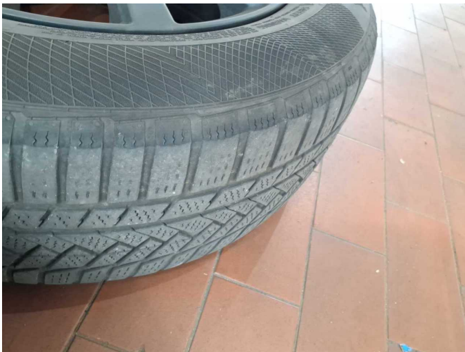
Damage 6: Wheel / tyres: Tyre - front - Abrasion - Replace
