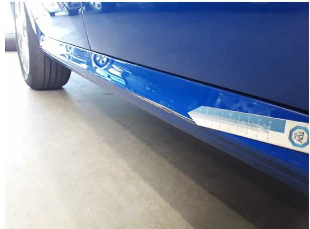
Damage #5: Sill - right side: Sill - Deformed - Repair and paint
