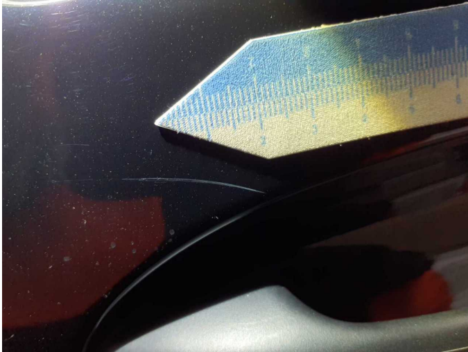
Damage 5: Sliding door - left side: Sliding door - Scratch(es) - Smart repair
