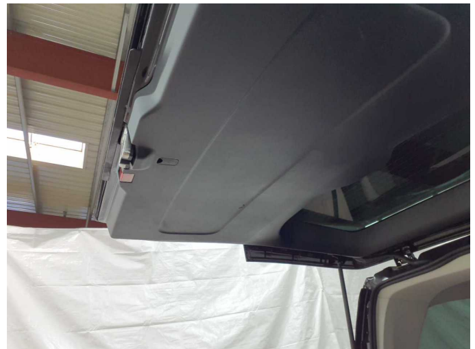
Damage 4: Boot lid / rear door: Trim - standard - lower - Scratch(es) - Loss in value
