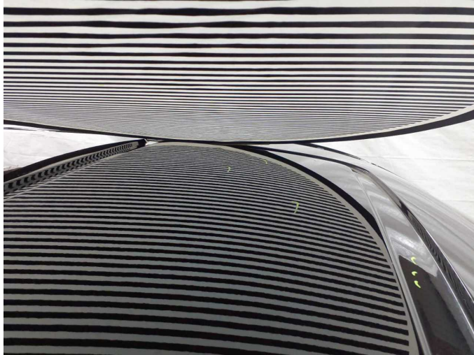
Damage 15: Roof: Roof (Anätzung) - Damage by hail - Repair and paint
