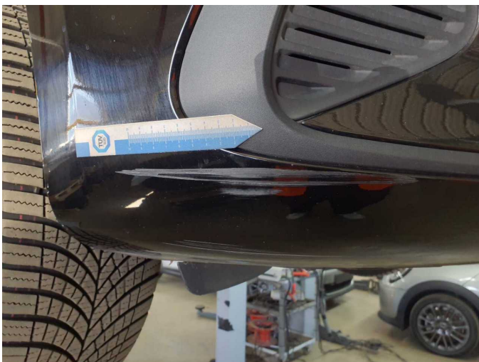
Damage 12: Front bumper: Front bumper - Scratched - Paint
