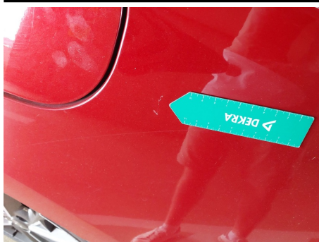
Kotflügel / Hinten Links / Delle
