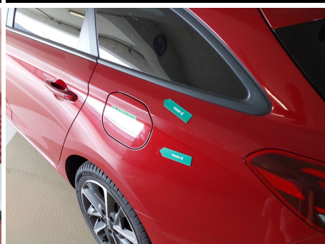
Kotflügel / Hinten Links / Delle
