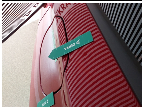
Kotflügel / Hinten Links / Delle
