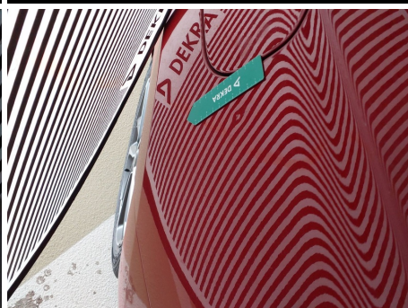
Kotflügel / Hinten Links / Delle
