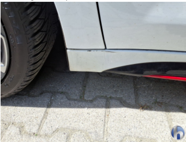
5. Schweller - Links Kratzer - Smart Repair
