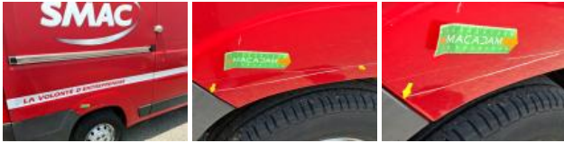
Outer sill R, Scratch(es), Paint
