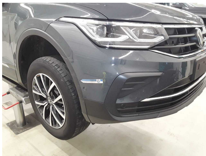
Damage 3: Front bumper: Front bumper (Incl. Anbauteile erneuern) - Scratched - Repair and paint
