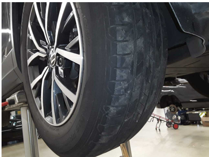
Damage 1: Wheel / tyres: Tyre - front - does not meet manufacturer specifications - Replace
