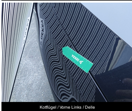
Kotflügel / Vorne Links / Delle
