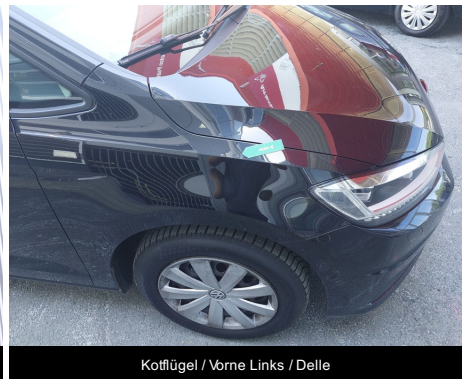
Kotflügel / Vorne Links / Delle
