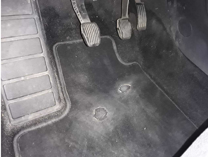
Damage 2: Trim / covers: Carpet - front left side - Broken / torn - Replace
