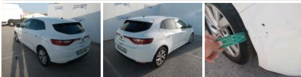
Bumper R, Scratch(es), Repair and paint (complete)
