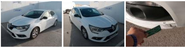
Bumper F, Broken, Repair and paint (complete)
