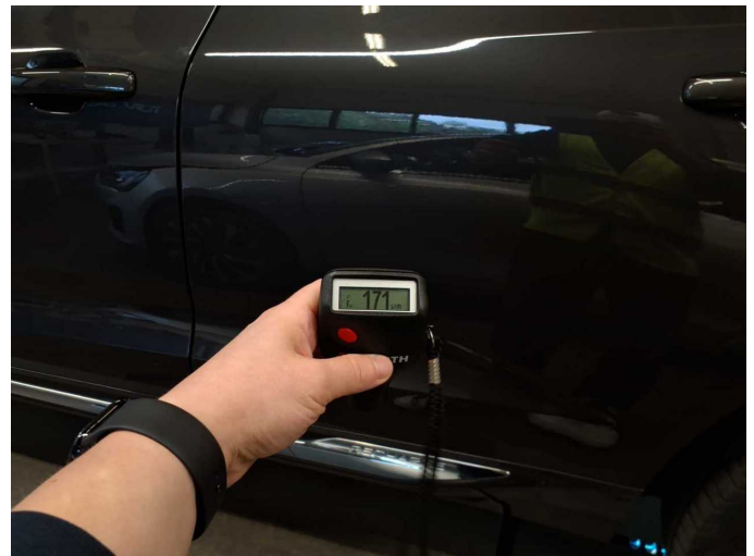
Repainting 1: Door - rear left side
