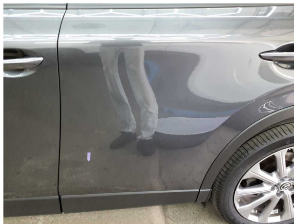
Beschädigung #4: Tür hinten links: Tür - Kratzer - Smart Repair
