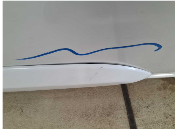
Damage #1: Door - rear left side: Brightware - lower - Malposition - Un- / install
