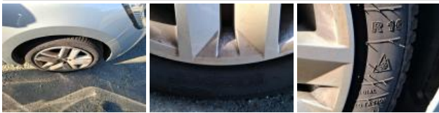
Tyre RR, Out of tolerance, Replace
