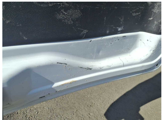
Damage 2: Boot lid / rear door: Rear door - left side (Innenseite) - Scratched - Smart repair
