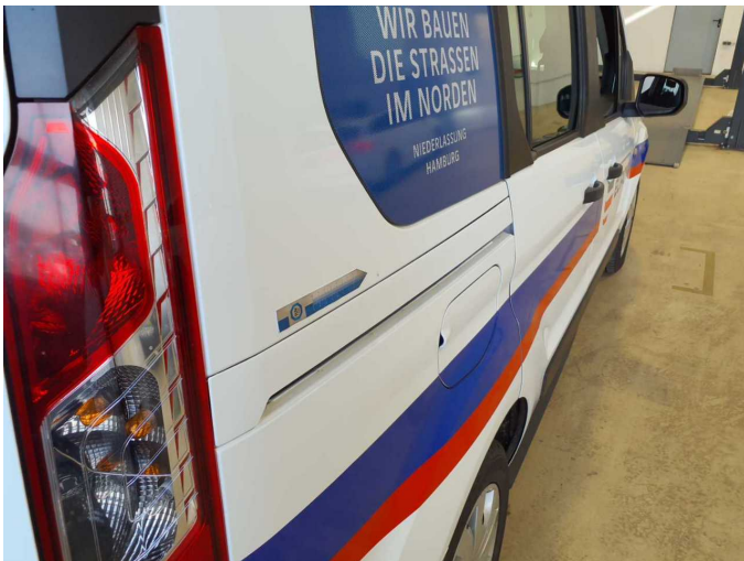
Damage 9: Side panel - rear right side: Side panel - Dent / paintcoat damage - Smart repair
