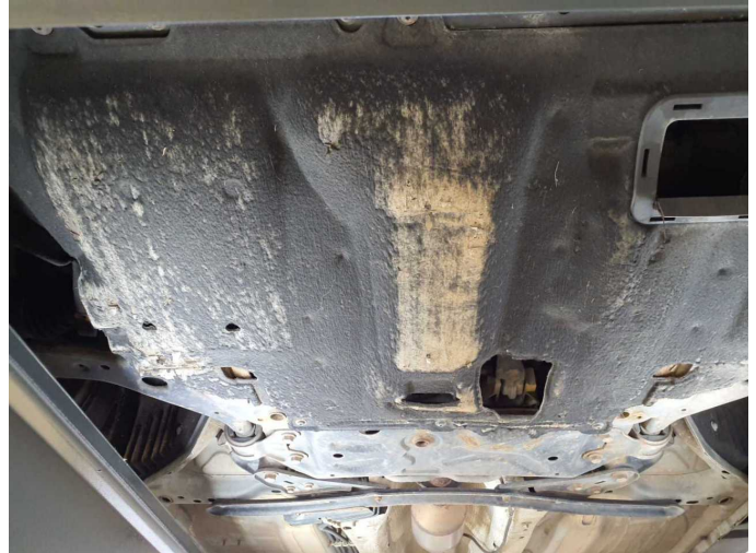
Damage 8: Body: Underbody panelling - Scratch(es) - Loss in value
