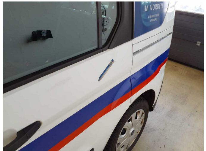
Damage 3: Sliding door - left side: Sliding door - dent(s) - Smooth repair work
