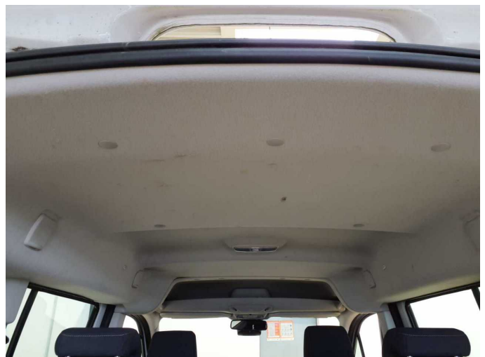
Damage 11: Trim / covers: Roof lining - Scratch(es) - Smart repair
