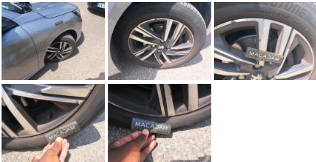
Tyre RR, Out of tolerance, Replace
