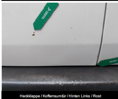
Heckklappe / Kofferraumtür / Hinten Links / Rost
