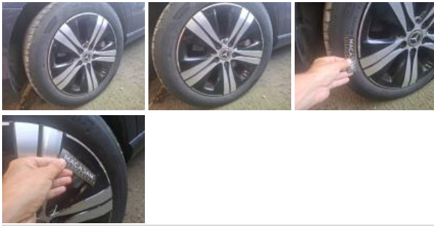
Tyre RR, Out of tolerance, Replace
