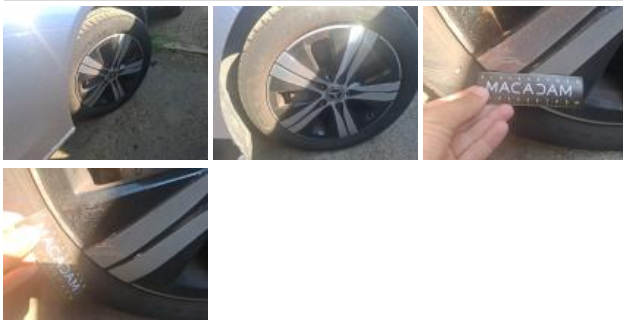
Tyre FR, Out of tolerance, Replace
