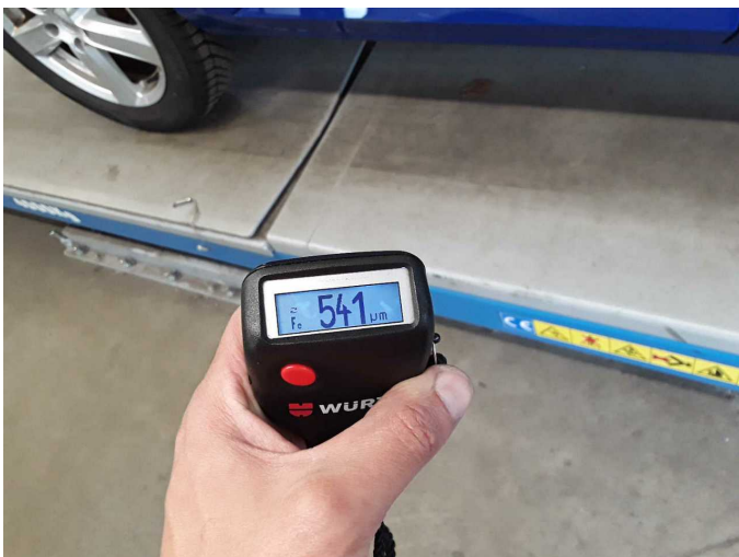
Repainting 1: Boot lid / rear door, Mudguard - right side, Side panel - rear right side, Door - rear right side, Door - front right side
