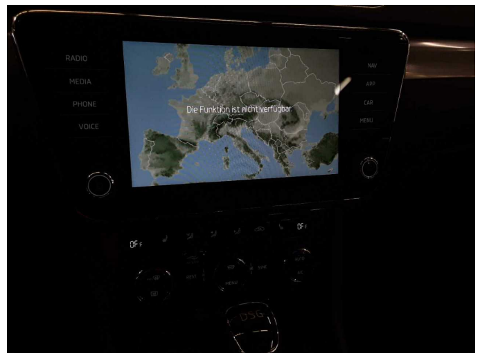
Missing part 1: Multimedia system: Navigation data storage - Missing - Replace
