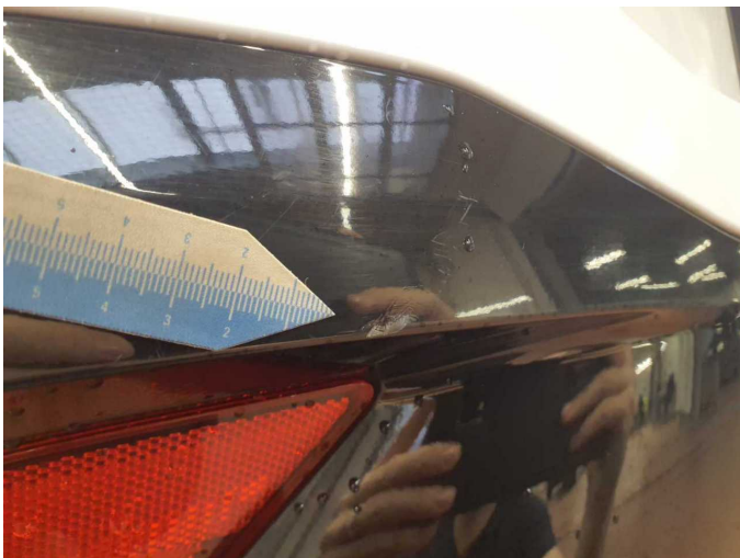
Damage 9: Rear bumper: Spoiler - Scratch(es) - Replace
