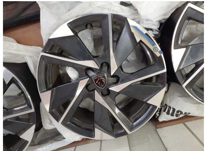
Damage 10: 2nd wheel set: 3 alloy rims - Scratched - Replace
