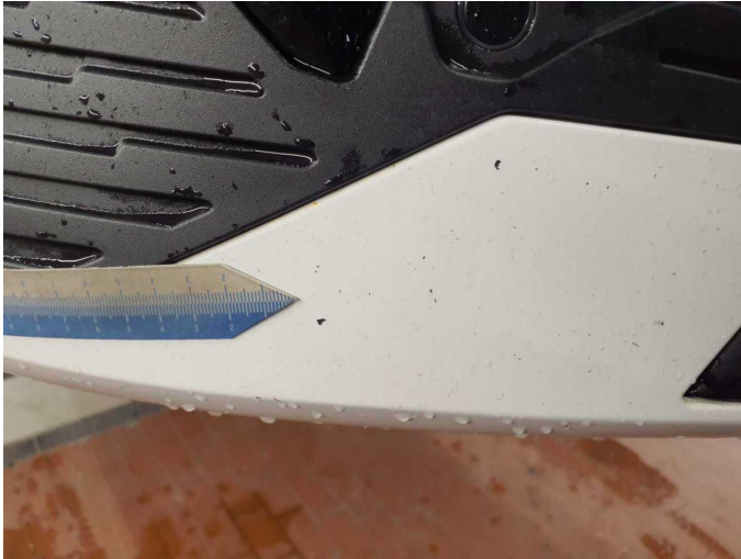
Damage 8: Front bumper: Front bumper - Scratched - Paint
