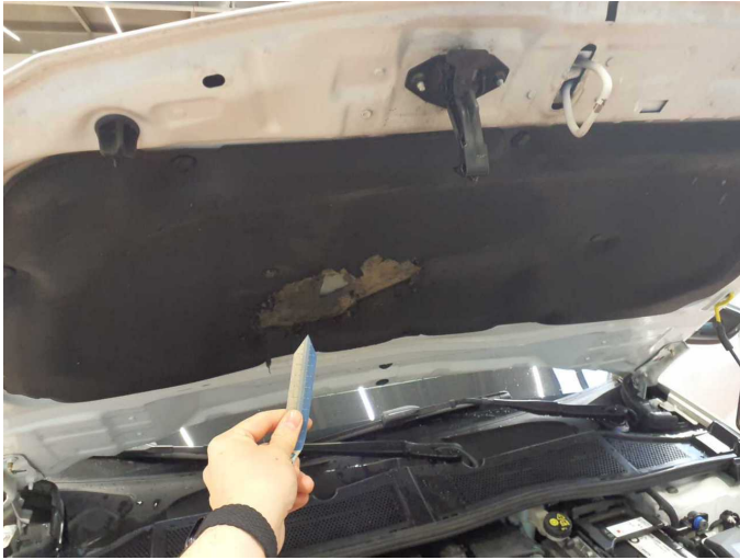
Damage 5: Bonnet: Insulation lining - Broken / torn - Replace
