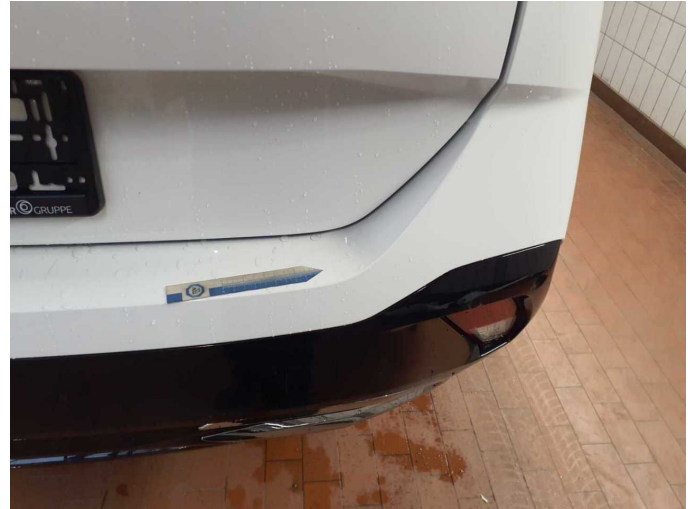
Damage 7: Rear bumper: Rear bumper - Scratch(es) - Paint
