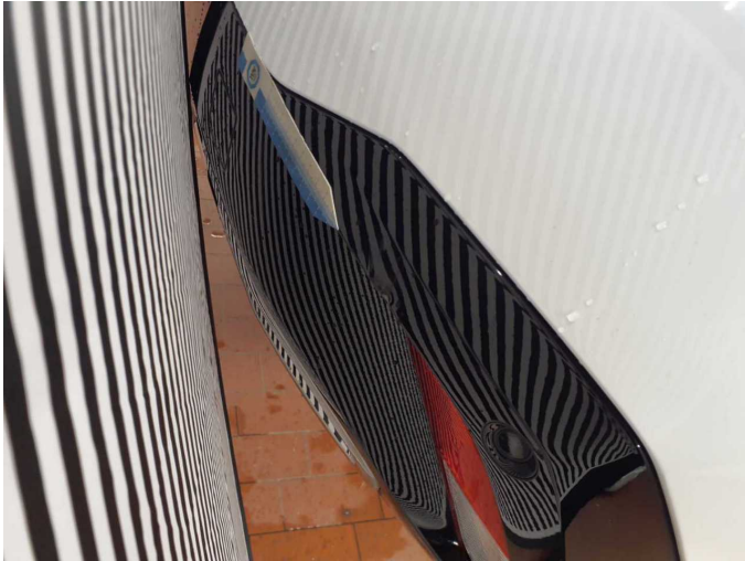
Damage 9: Rear bumper: Spoiler - Scratch(es) - Replace
