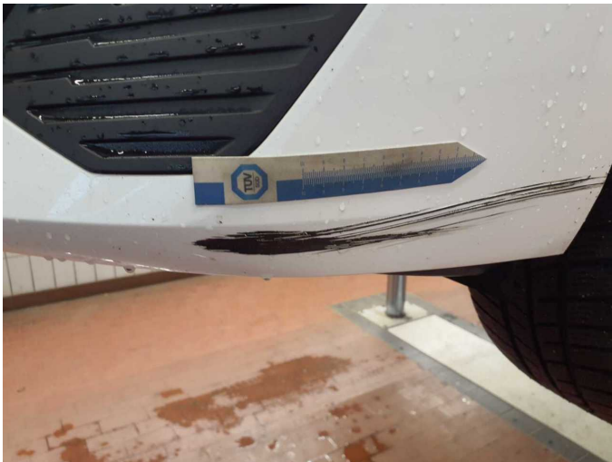
Damage 8: Front bumper: Front bumper - Scratched - Paint
