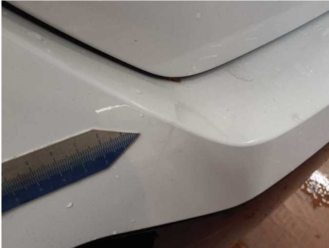
Damage 7: Rear bumper: Rear bumper - Scratch(es) - Paint
