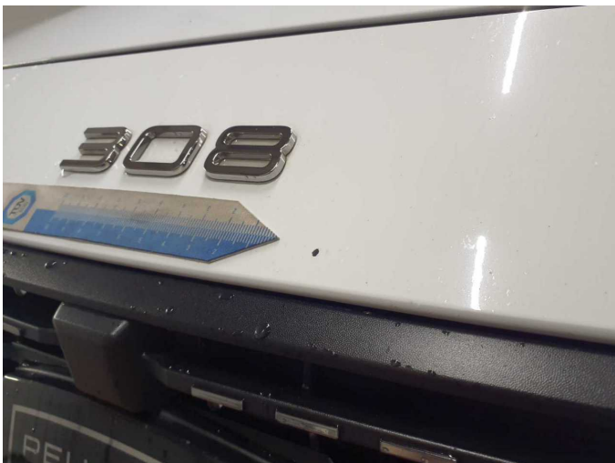
Damage 8: Front bumper: Front bumper - Scratched - Paint
