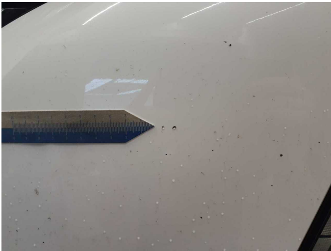
Damage 8: Front bumper: Front bumper - Scratched - Paint
