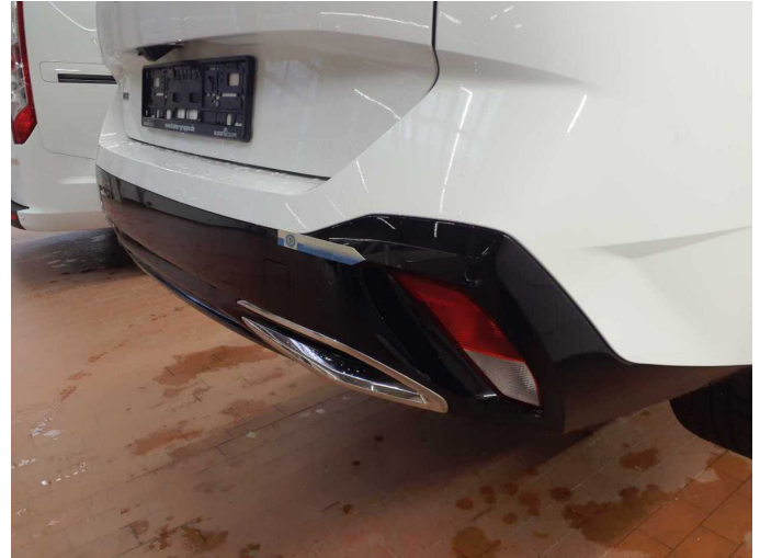
Damage 9: Rear bumper: Spoiler - Scratch(es) - Replace
