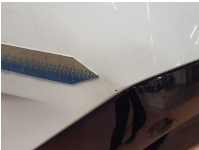
Damage 7: Rear bumper: Rear bumper - Scratch(es) - Paint
