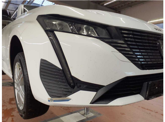
Damage 8: Front bumper: Front bumper - Scratched - Paint
