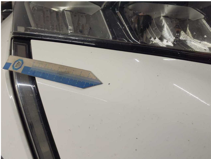
Damage 8: Front bumper: Front bumper - Scratched - Paint
