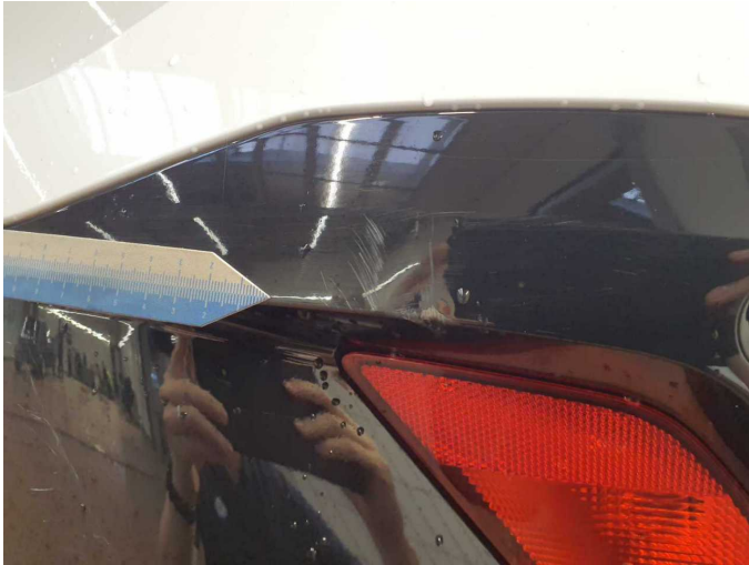
Damage 9: Rear bumper: Spoiler - Scratch(es) - Replace
