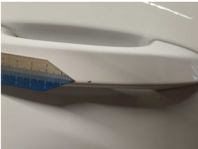
Wear and tear 2: Door - front right side: Door handle - outside - Scratch(es) - No deduction
