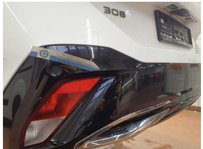
Damage 9: Rear bumper: Spoiler - Scratch(es) - Replace
