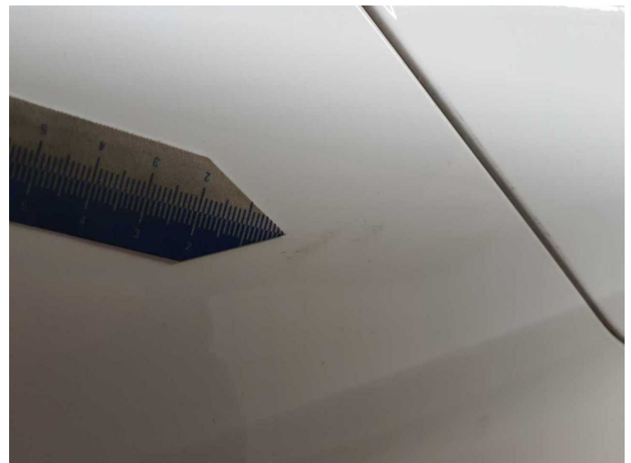
Damage 7: Rear bumper: Rear bumper - Scratch(es) - Paint
