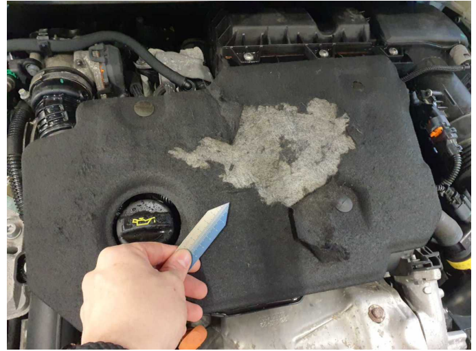
Damage 6: Engine: Engine cover - Broken / torn - Replace
