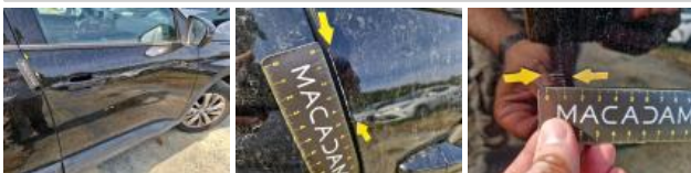
Door RR, Dent(s), Repair and paint (complete)
