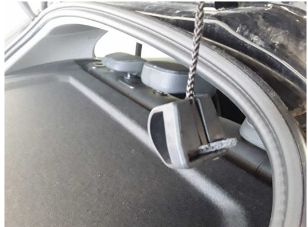
Damage #4: Interior: Rear shelf - Broken / torn - Replace
