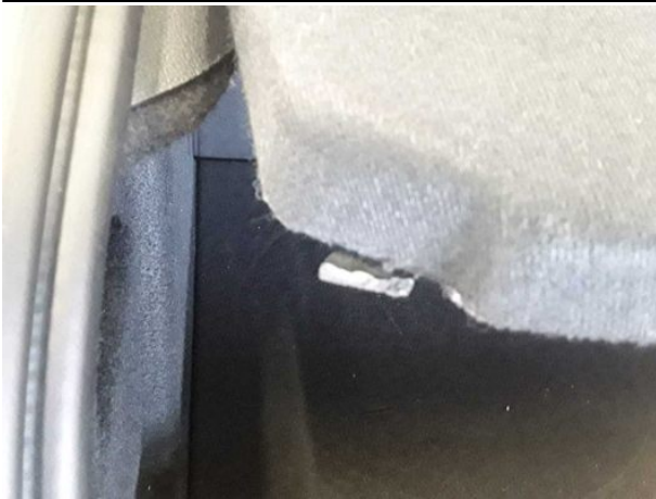
Damage #4: Interior: Rear shelf - Broken / torn - Replace
