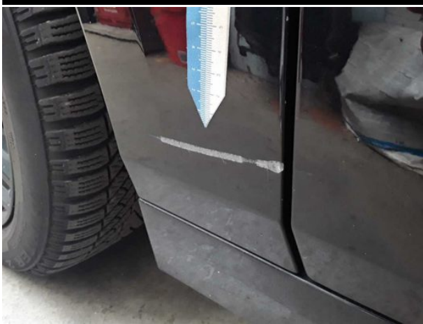
Damage #8: Mudguard - left side: Mudguard - left side - Scratch(es) - Repair and paint
