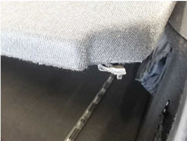
Damage #4: Interior: Rear shelf - Broken / torn - Replace
