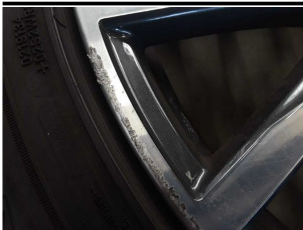
Damage #5: 2nd wheel set: 3 alloy rims - Scratched - Loss in value
