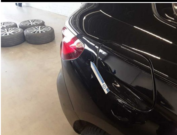
Damage #6: Side panel - rear right side: Side panel - Scratched - Paint
