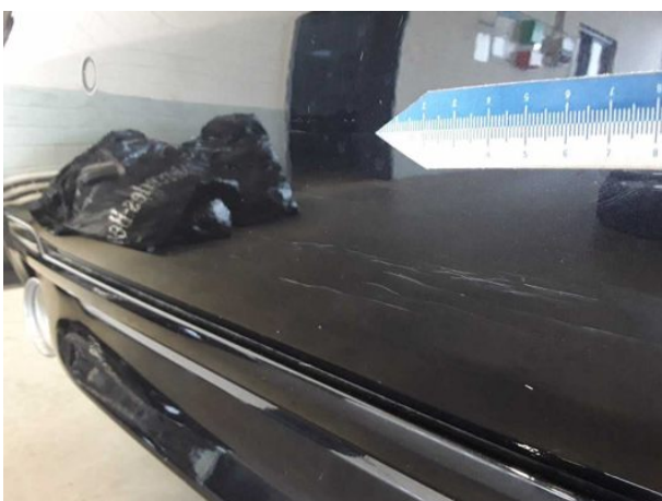
Damage #7: Rear bumper: Rear bumper - Scratched - Paint
