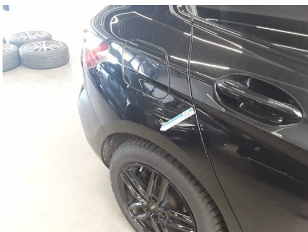
Damage #6: Side panel - rear right side: Side panel - Scratched - Paint
