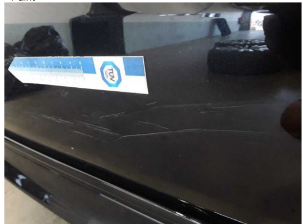
Damage #7: Rear bumper: Rear bumper - Scratched - Paint
