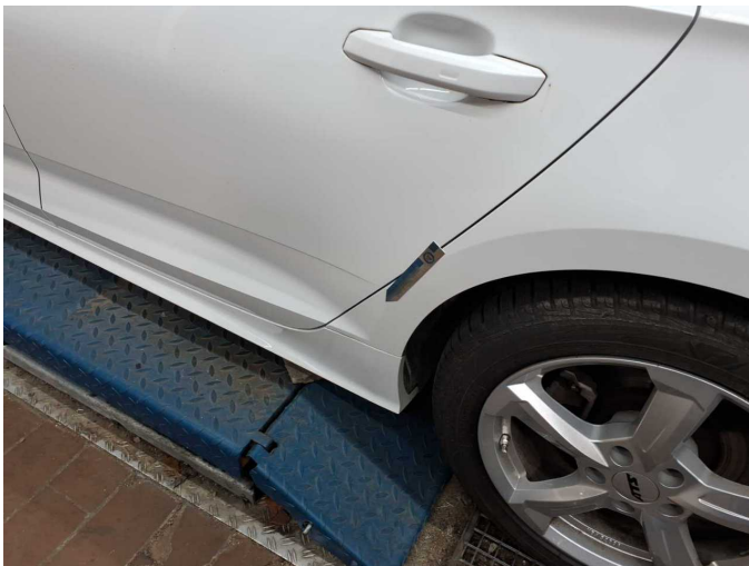
Damage 2: Side panel - rear left side: Elbow - dent(s) - Smooth repair work
