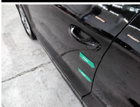
Tür / Vorne Links / Kratzer
