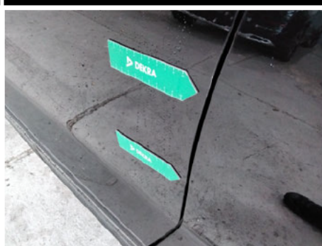
Tür / Vorne Links / Kratzer
