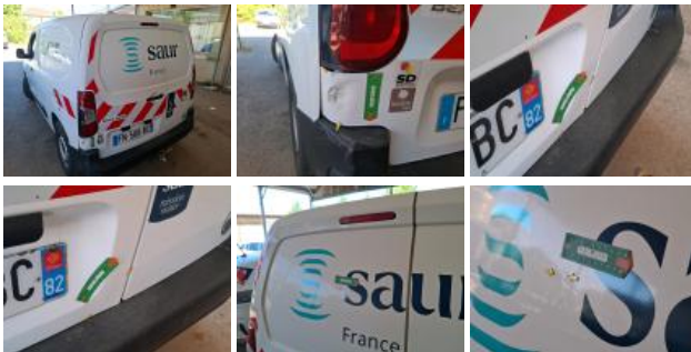
Bumper R, Deformed / Strained, Replace
