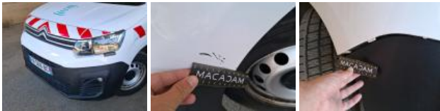
Bumper F, Broken, Replace
