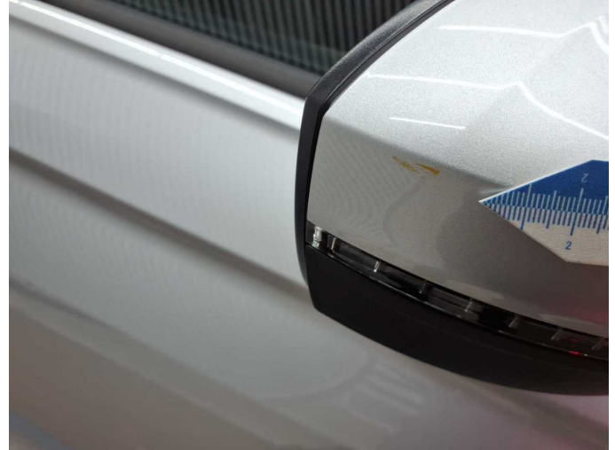
Wear and tear 3: Wing mirror - right side: Cap (polierbar) - Abrasion - No deduction
