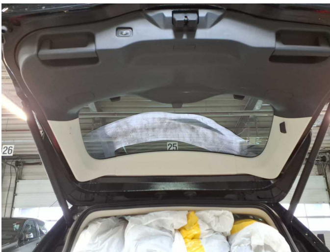
Damage 3: Trim / covers: Boot lid - interior trim (Halter) - Missing - Repair
