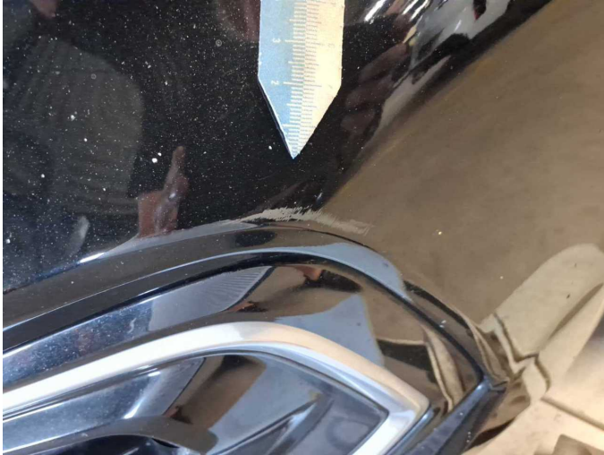
Damage 15: Front bumper: Front bumper - Scratched - Paint
