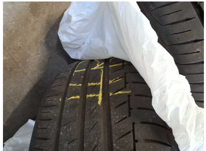
Damage 11: 2nd wheel set: 1 tyre (Flanke) - Damaged - Replace
