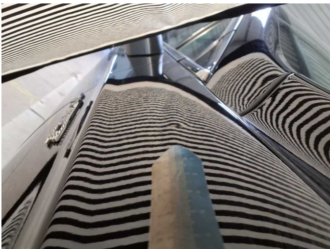
Wear and tear 4: Mudguard - right side: Mudguard - right side - dent(s) - Smooth repair work
