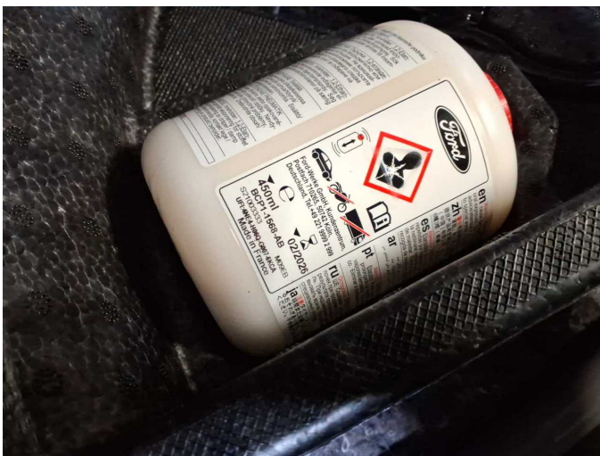
Damage 4: Equipment: Tirefit filler - Expired - Replace
