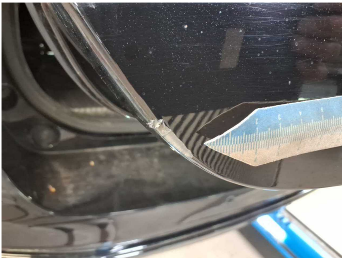
Damage 10: Boot lid / rear door: Boot lid - Scratch(es) - Smart repair
