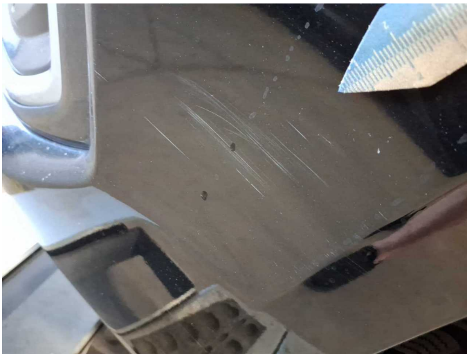
Damage 15: Front bumper: Front bumper - Scratched - Paint
