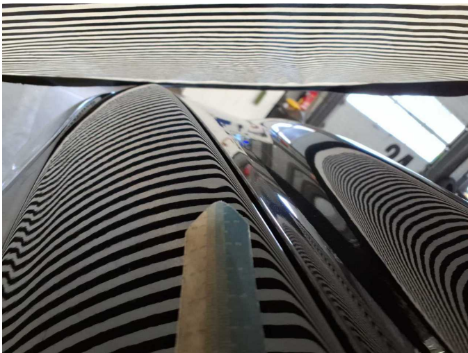
Wear and tear 3: Mudguard - left side: Mudguard - left side - dent(s) - Smooth repair work
