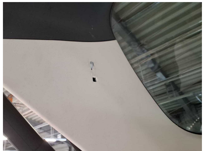
Damage 3: Trim / covers: Boot lid - interior trim (Halter) - Missing - Repair
