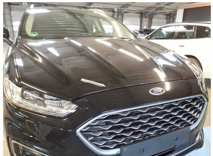
Damage 17: Bonnet: Bonnet (Dellen) - Corrosion - Repair and paint
