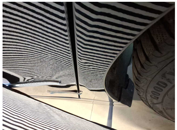
Damage 9: Side panel - rear left side: Side panel - dent(s) - Smooth repair work
