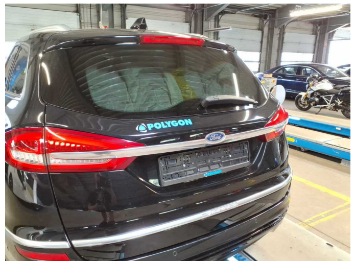
Damage 5: Body: Body - Glued / labelled - De-glue / neutralise
