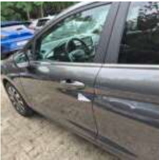
Damage Part Frontdoor – Left
