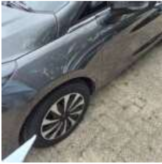
Damage Part Wheelcover - Left Front
