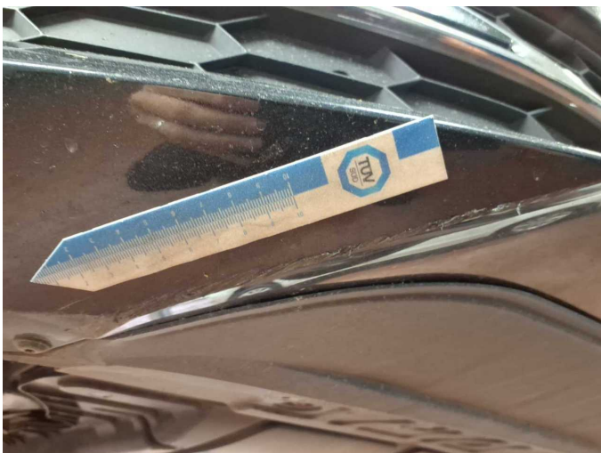
Damage 5: Front bumper: Front bumper - Deformed - Repair and paint
