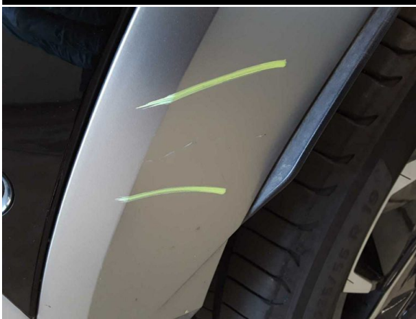
Damage #4: Mudguard - right side: Wheel well extension - Scratched - Smart repair
