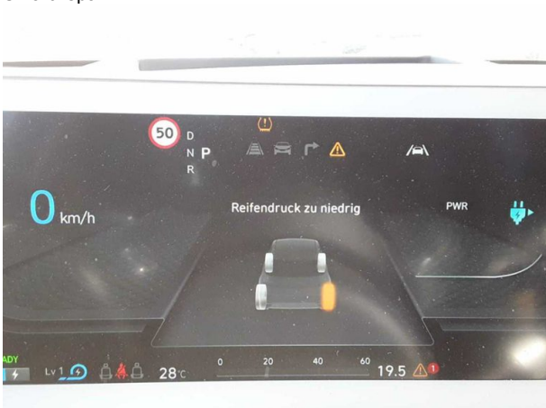
Damage #6: Instrument panel: Indicator light (RDKS leuchtet) - Specify findings - Diagnosed and repair if necessary
