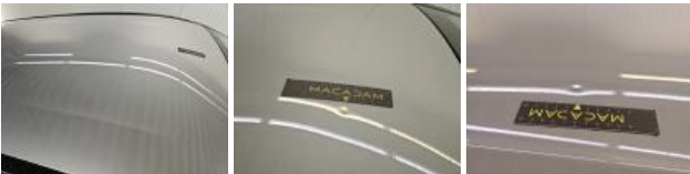
Roof, Dent(s), Paintless dent repair
