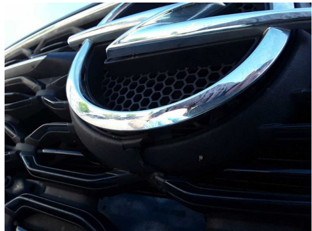
Damage #2: Front structure: Emblem (Lose) - Damaged - Replace
