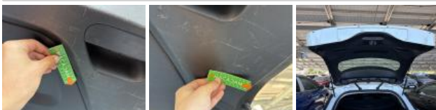
Boot lid covering R, Scratch(es), Replace
