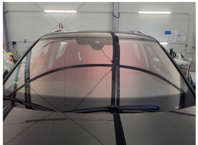
Damage 1: Vehicle glazing: Windscreen with lane departure assistant - Broken / torn - Replace
