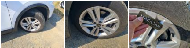
Tyre FL, Tear, Replace
